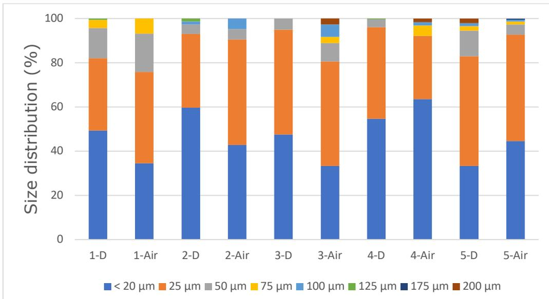
Figure 9. Size distribution of microplastics (%) in both deposited (D) and airborne (Air) samples of all study sites.
