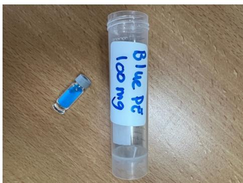
Figure 3. Blue Polyethylene (PE) used for spiking the Quartz filter.
