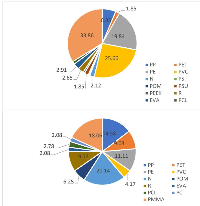
Figure 8. Relative frequency distribution of polymers (%) amongst deposited (top picture) and airborne (bottom picture) samples.
