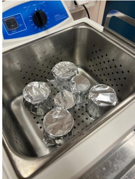
Figure 5. Extraction of microplastic from quartz filters, placing the filter in a glass beaker (top left), vertexing the beakers (top right), and ultrasonic bath (bottom).
