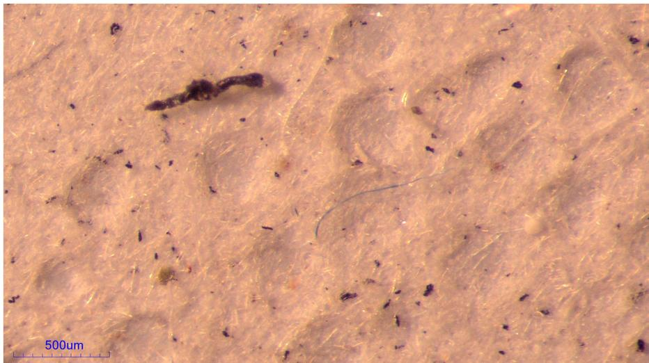
Figure 7. Discrimination between natural and synthetic fiber under microscope (40x). The black fiber is natural, but the thin blue fiber is synthetic. Picture is from one of the deposited dust samples collected at the secondhand clothing shop in Utrecht on 31 August 2022.
